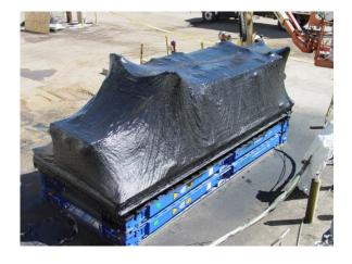
The radioactive/beryllium contaminated press in these photos was packaged using this system.
