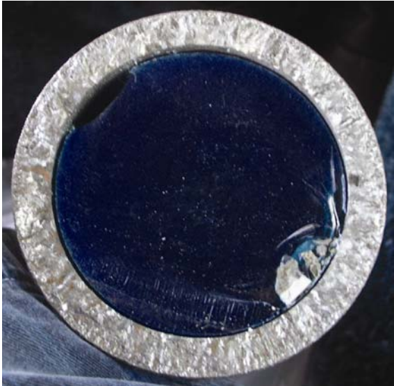
CC PS 413 in 4-inch Dur-Iron pipe
